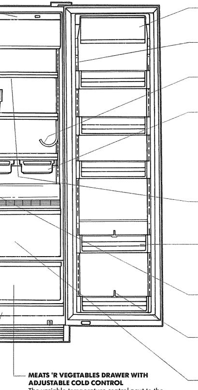
The variable temperature control next to the Meats 'R Vegetables drawer regulates the flow of cold air from the freezer. Set the control lever all the way down to the coldest setting to store meats. Set it
